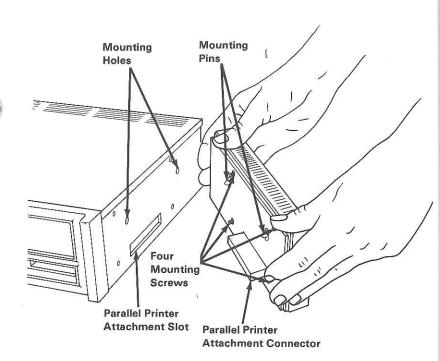
Install the option attachment cover. Make sure it is pressed firmly into the mounting holes.
